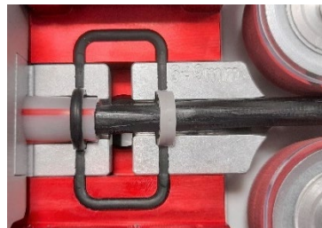
Figure 19: positioning the gaskets with cut facing down
