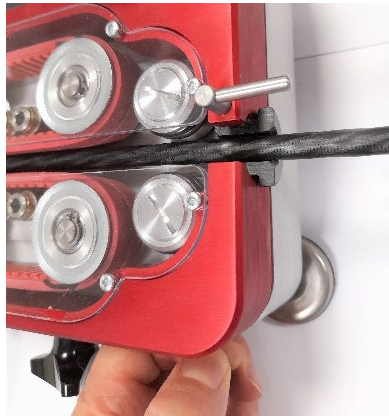
Figure 20: pulling the meter counter wheel opening lever to insert the cable
