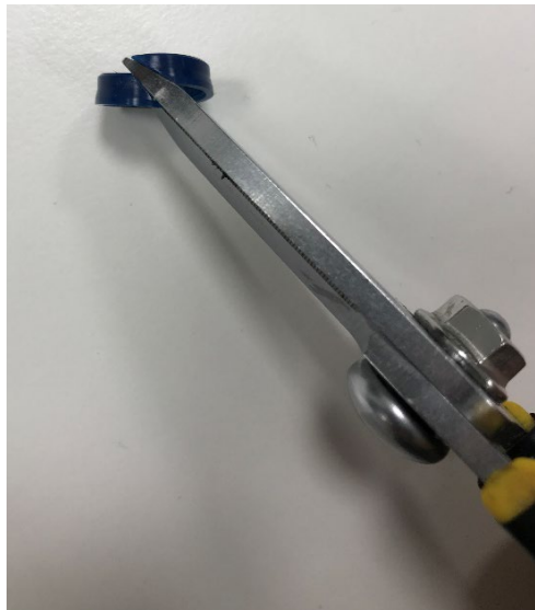
Figure 17: cut gaskets diagonally.
