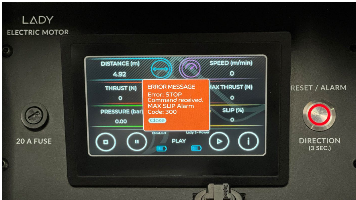
Figure 10: STOP Command Received error. MAX SLIP Alarm
