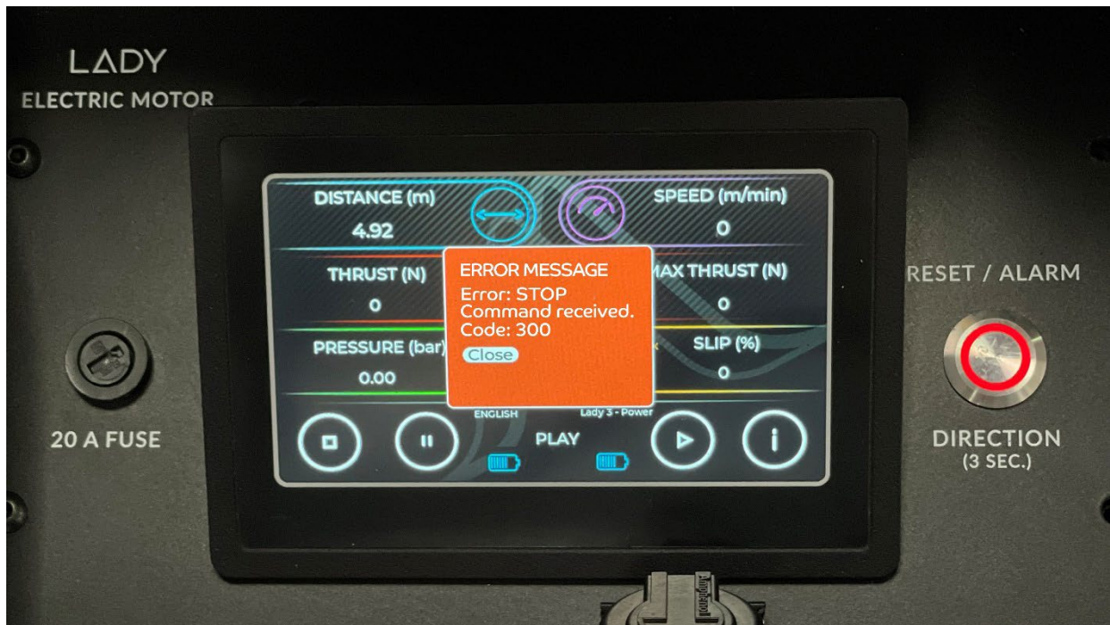
Figure 9: STOP Command Received error.
