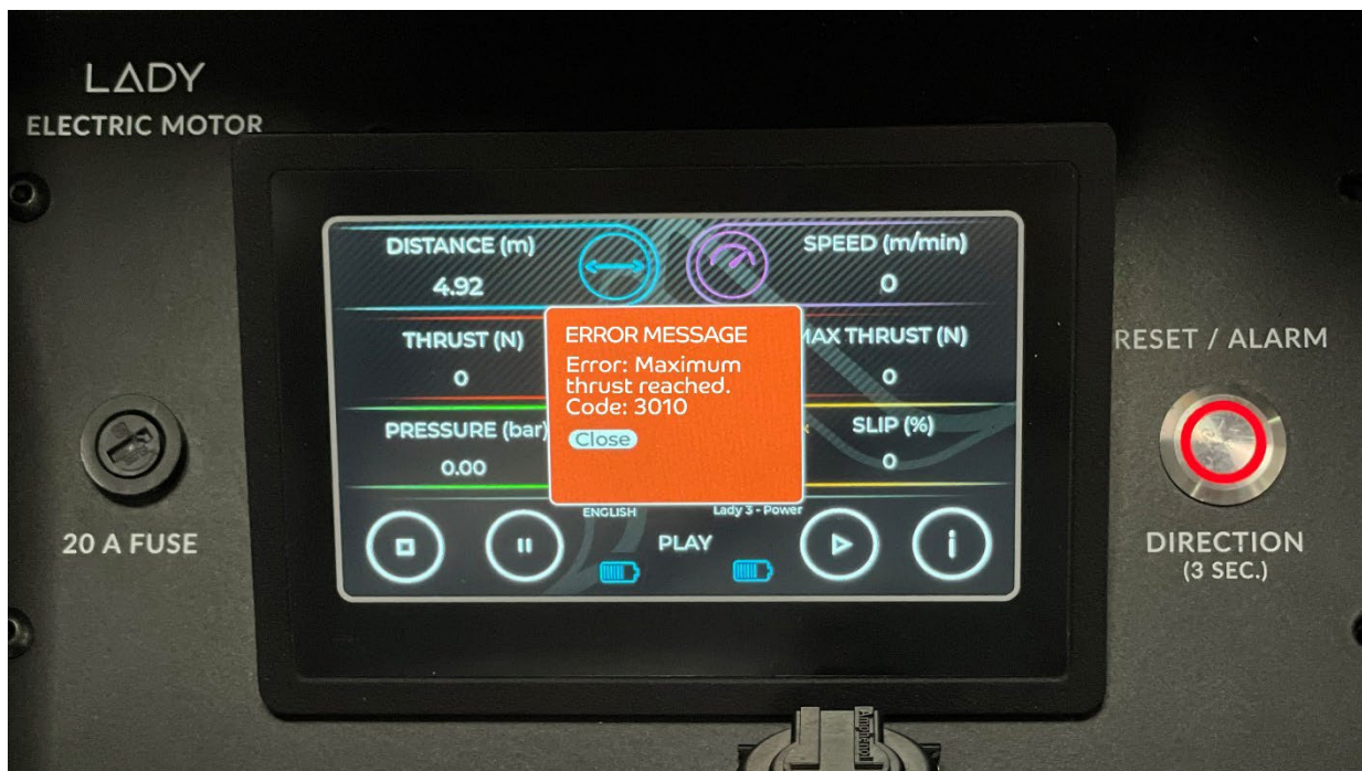
Figure 8: Maximum Thrust Reached error.
